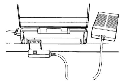
When you are not using the AC adapter, replace the safety cover that protects the connector.
